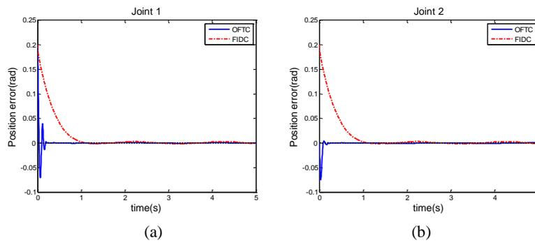
Figure 4. Tracking error
